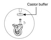
3. Carefully place the serving / transport trolley on the floor and make sure that all swivel castors touch the surface. The serving / transport trolley may be aligned by adjusting swivel castors. Secure their position with lock nuts.
